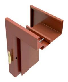
Steel adjustable frames are designed for installation in various types of rooms with finished walls and floors, including flats, public buildings, hotels, etc. The complete frame kit consists of a main section, adjustment part, with a seal, hinges and a set of plugs also included.
