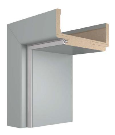
The DUALE adjustable frame is made of MDF to any wall thickness, starting at 100 mm. Four-centimetre adjustment is provided in the form of an adjustable angle bracket. The frame can also be manufactured to any clear width. The complete frame consists of two side jambs and a head jamb with angles on both sides.
