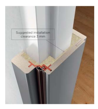
The Steel Frame Casing is a solution which lets you forget about problems related to non-standard hinge spacing in the existing frame, non-standard strike plate positions or sizes, and very common non-standard rebate (lip) dimensions. To complete a quick and hassle-free installation on the existing frame, you only need to remove the existing hinges, but only if they protrude beyond the outline of the lining.
